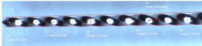
Figure 2: Micromorphometry photography. The diameters of the instruments.
